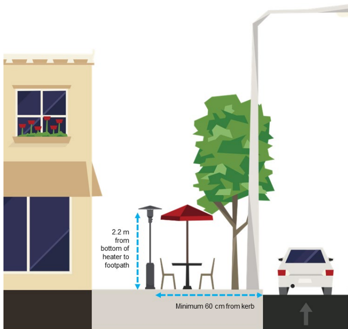
Figure 4 – Gas heaters can only be installed or placed within the trading zone. They must sit at least 60cm from the kerb, and the bottom of the heater must sit at least 2.2 m above the footpath.
